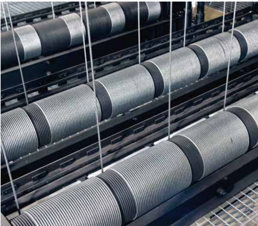
The scenery is moved simultaneously using four winches with amazing cable control, using a battery-powered drive and, in another stage of expansion, using an electric drive.
