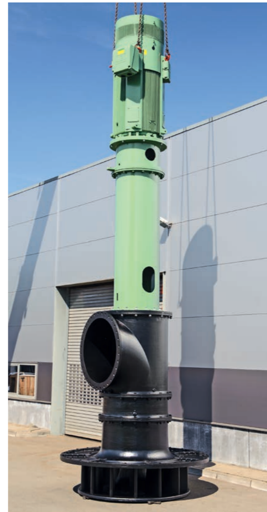
Large pump for the pump station Dahme VP 1200 vertical propeller pump 4,000 l/s 3.4 m 220 kW
